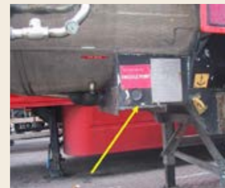
Fig no. 11 Example of a suitable trestle points on a tank unit.
